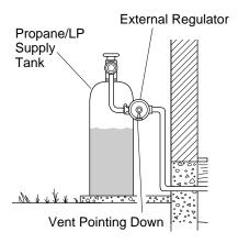
Figure 13 - External Regulator With Vent Pointing Down
